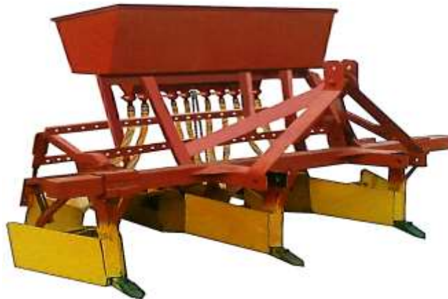
Figure 2: Machine for rainwater harvesting and planting the wheat crop.
