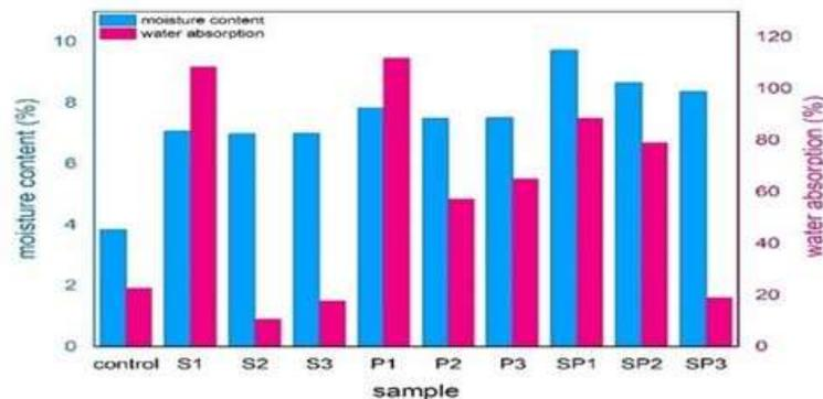
Figure 4: Moisture content and water absorption of biofoams
