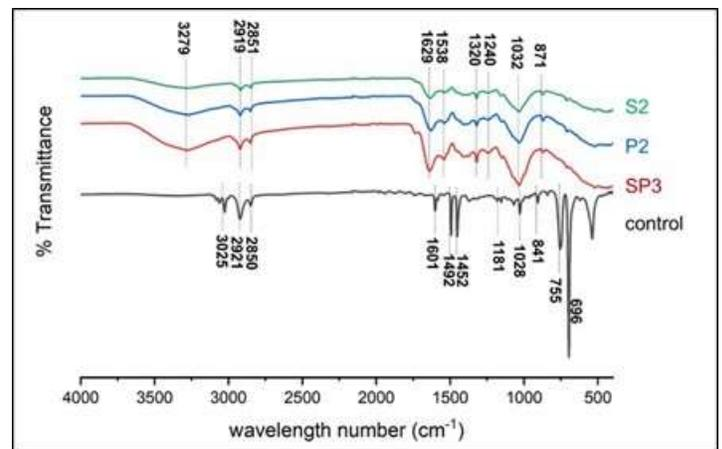
Figure 7: FTIR spectra of biofoams and styrofoam as control
