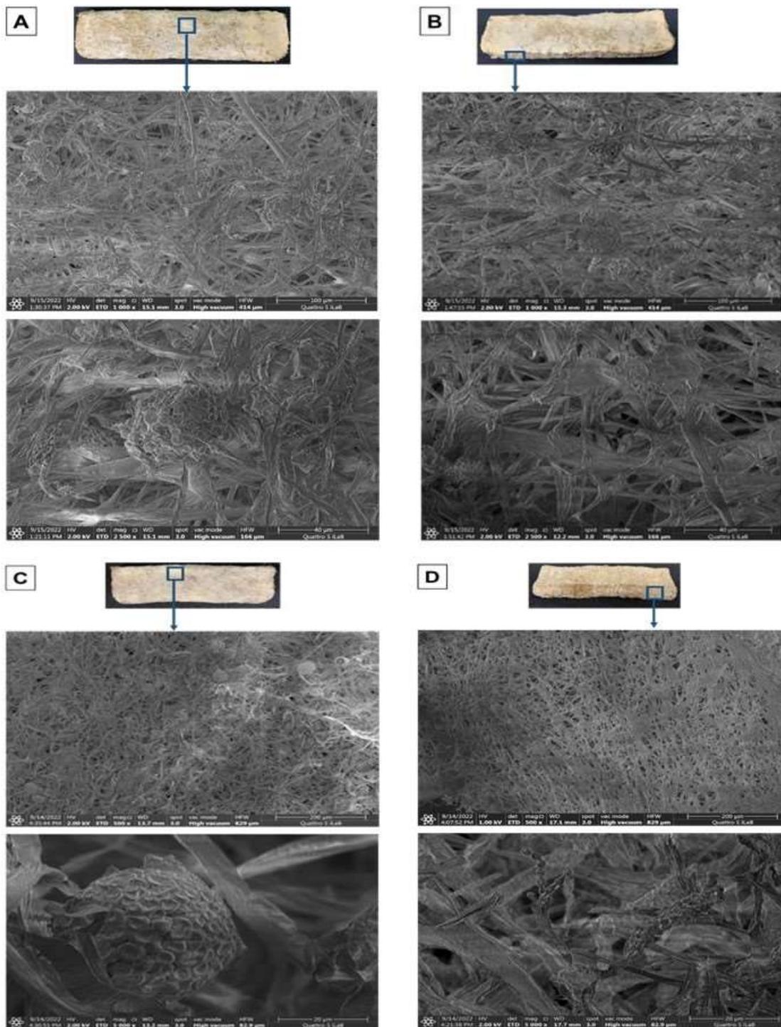
Figure 5: Morphology of biofoam using FESEM: A) surface of S2, B) cross section of S2, C) surface of P2, and D) cross section of P2.
