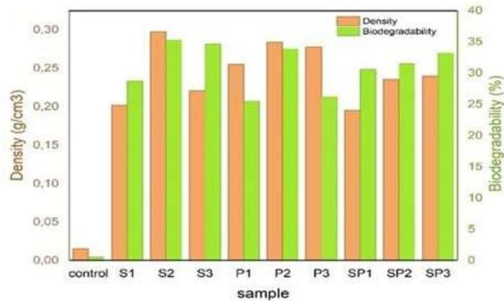
Figure 3: Density and biodegradability of biofoams
