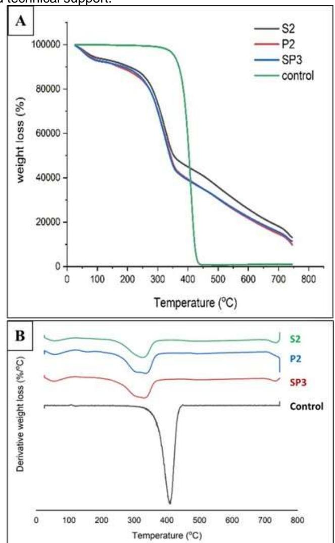
Figure 8: TGA analysis of biofoam. A) weight loss, B) derivatives weight loss.
