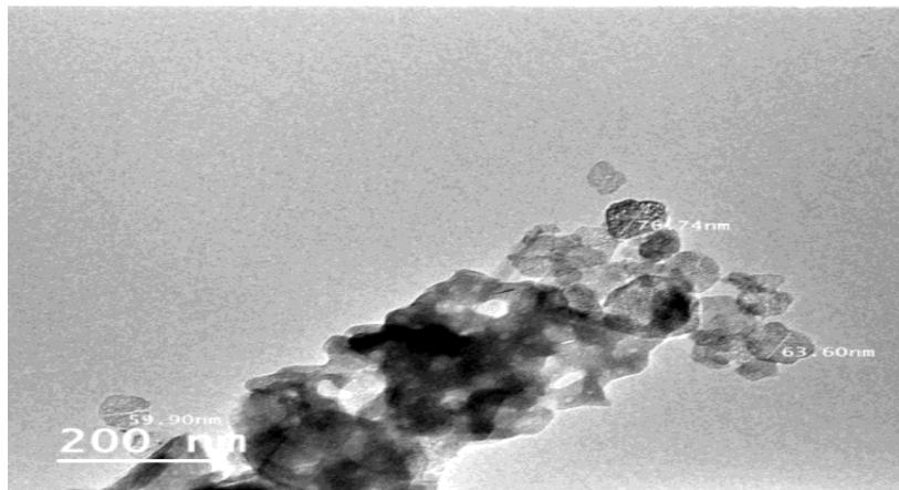
Figure 3. Scanning by electron microscopy for nano-imidacloprid at 200 nanometer
