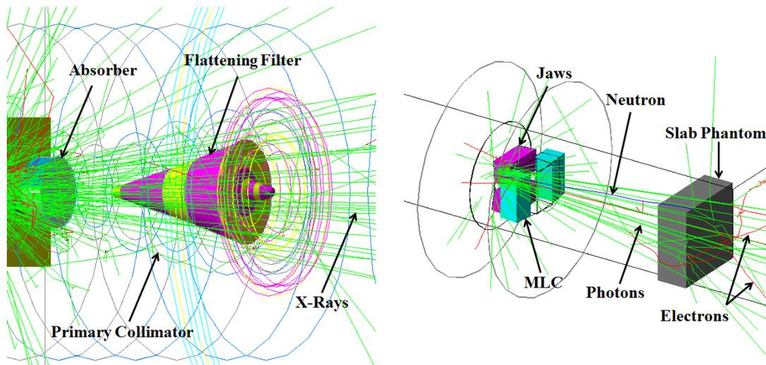
Figure 2: The stages of the simulation process: phase space (PhS) stage (Left), and dose calculation stage (Right).
