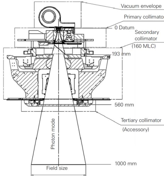
Figure 1: The main components of the Linac head.
