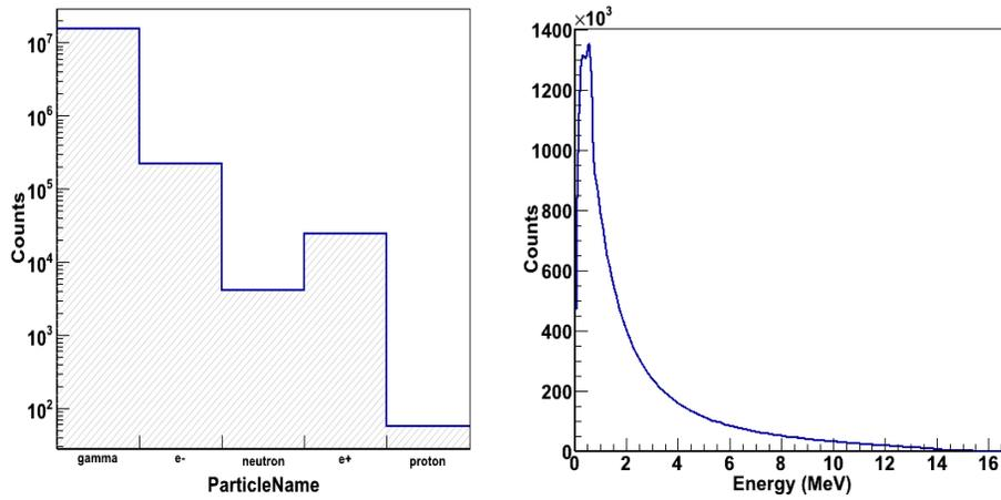
Figure 3: Particles types produced from the Linac head (Left), and photon spectrum (Right).
